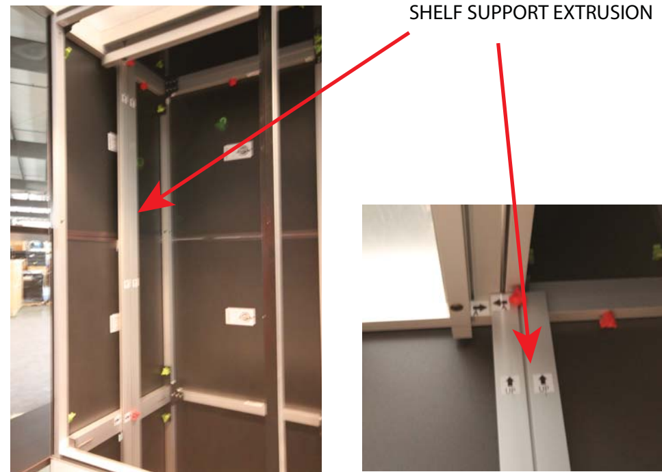
STEP 1: ATTACH THE SHELF SUPPORT EXTRUSION TO THE INSIDE OF THE LEFT-HAND 2X4 MAX FRAME USING THUMBSCREWS. SEE PHOTOS.
