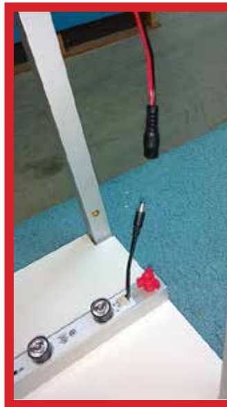
CONNECT TOP EXPOLIGHT BAR TO BOTTOM EXPOLIGHT BAR WITH RED AND BLACK COATED POWER CORD
