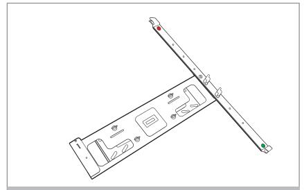
2 Attach the numbered (2) mount to the right side with provided thumbscrews as shown.
