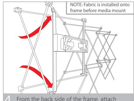
/ From the back side of the frame, attach media mount to REVERB frame as shown.
